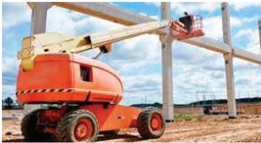
Boom Lift (45', two person) for parking lot light replacement & cleaning church stone walls.
